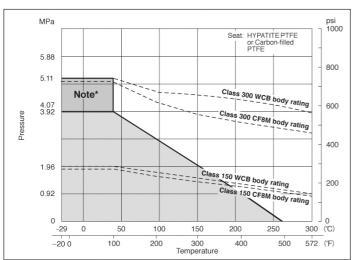
Note\*: Continuous pressurization is not recommended in this P-T range.
